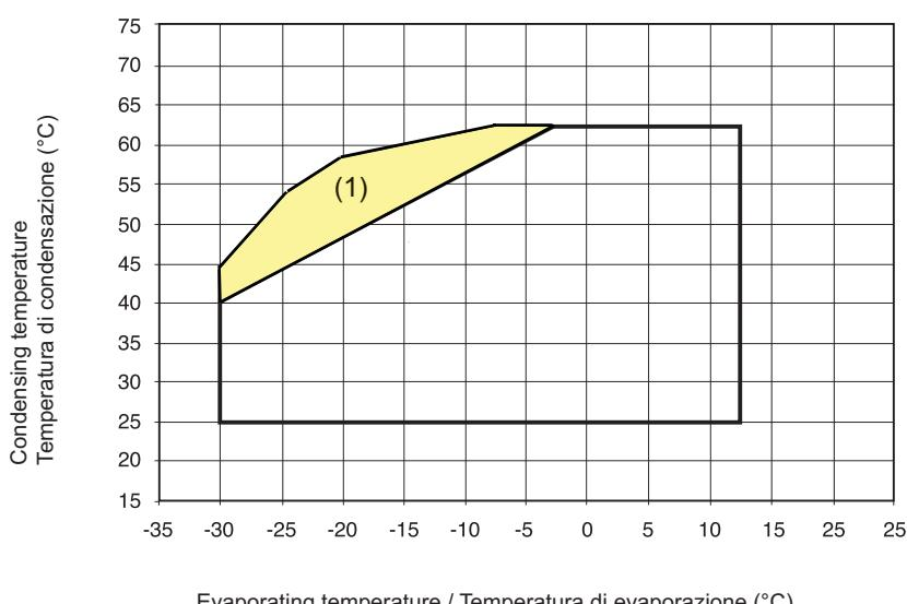
Zone n° 1 identifies working conditions requiring additional cooling of the compressor via liquid injection.
