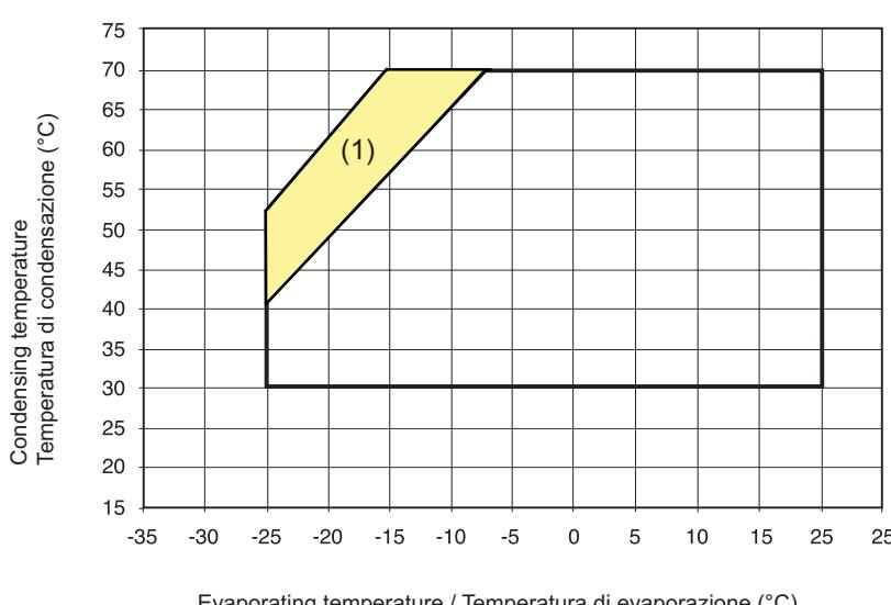
Zone n° 1 identifies working conditions requiring additional cooling of the compressor via liquid injection. The limits refer to 10K suction gas superheat. Higher superheat and part load operation may cause a restriction of the application limits (consult RefComp).
